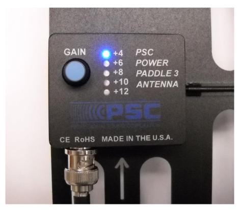
Gain settings are easily adjusted using the rotary switch. Gain setting is displayed by a lighted LED.
